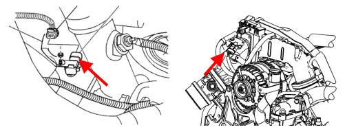
Figure 1 - '02-'04 (Left) and 04.5-09 (Right) MAP Sensor Locations
