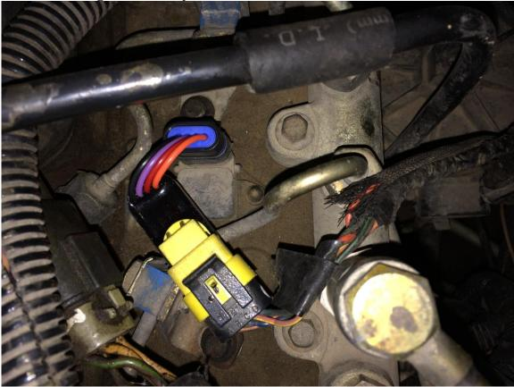
After you have plugged the factory harness into the yellow connector on the Boost Fooler you are done! As stated earlier the Boost Fooler was designed to be "Plug and Play" for a simple and fast installation.
