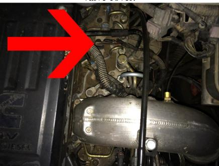
Here you can see the factory wiring harness and connector plugged into the MAP sensor
