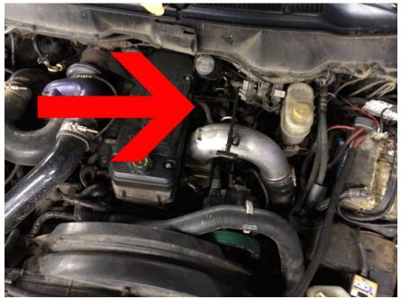
The sensor is located just behind the intake horn to the right of the valve cover.
