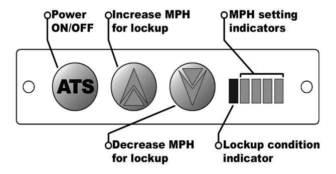
The ATS Co-Pilot will need to be set up for your vehicle and application. The Co-Pilot will need to be disassembled to access the dip switches on the electronic board. You will need a  $1/16^{th}$  - inch hex (Allen wrench) to remove the face from the Co-Pilot. After the face has been removed the electronic board can be slid out of the casing from the front. The digital face is attached to the circuit board with a ribbon
