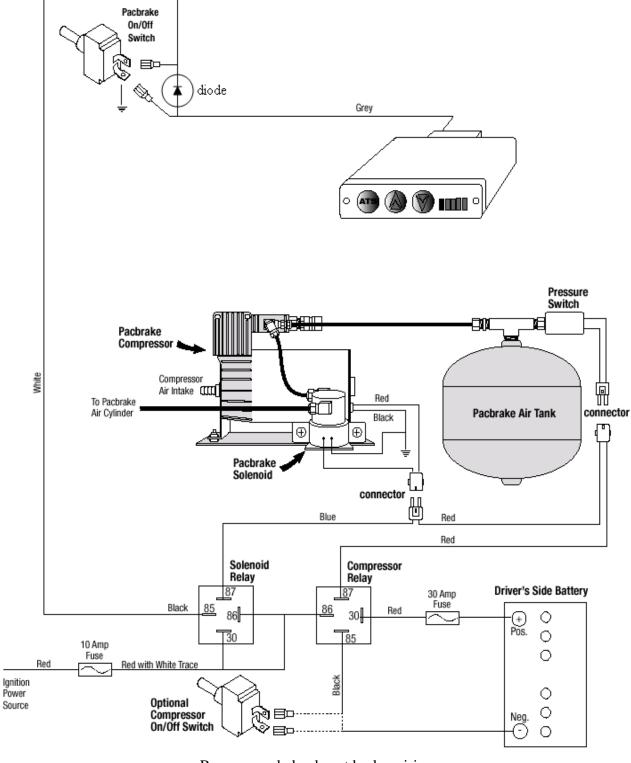
Recommended exhaust brake wiring
