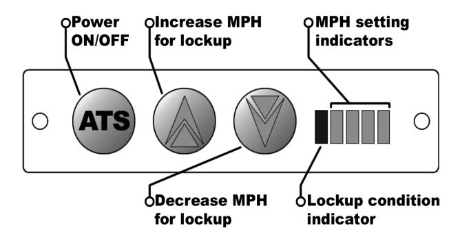
The ATS Co-Pilot will need to be set up for your vehicle and application. The Co-Pilot will need to be disassembled to access the dip switches on the electronic board. You will need a 1/16<sup>th</sup> - inch hex (Allen wrench) to remove the face from the Co-Pilot. After the face has been removed the electronic board can be slid out of the casing from the front. The digital face is attached to the
