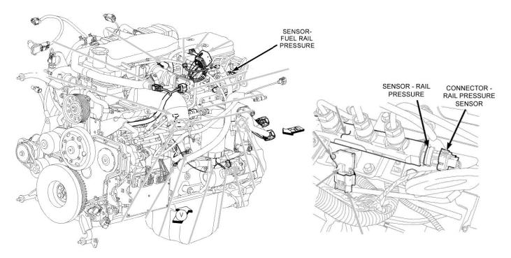
Figure 1 - Rail Pressure Sensor Location
