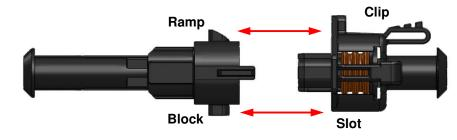
Figure 2 - Rail Pressure Sensor Connector Orientation
