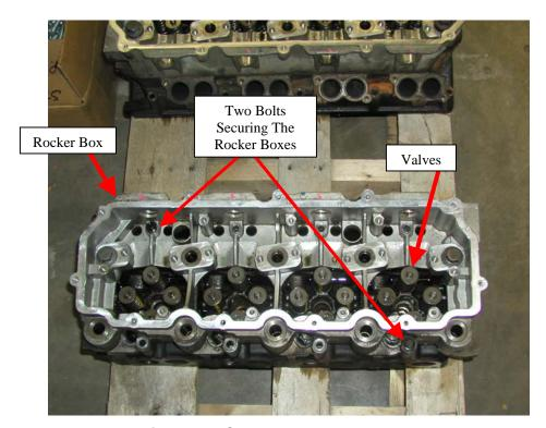
Figure 1: Correctly Prepared Heads
