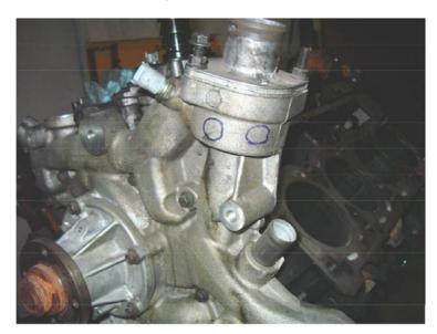
5. Drill pilot hole in desired location, progressively drill to a size of 7/16". Tap hole with 1/4-18" NPT tap. Install fitting with thread sealant. Repeat for second hole. Attach lines.
