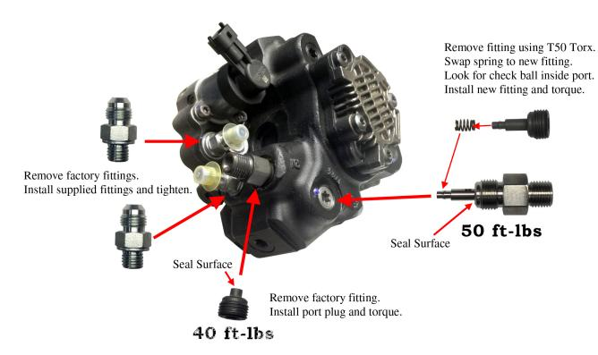
Note: A useful hint for installing the fittings is to install the pump on the pump bracket and clamp the bracket in a vice.
