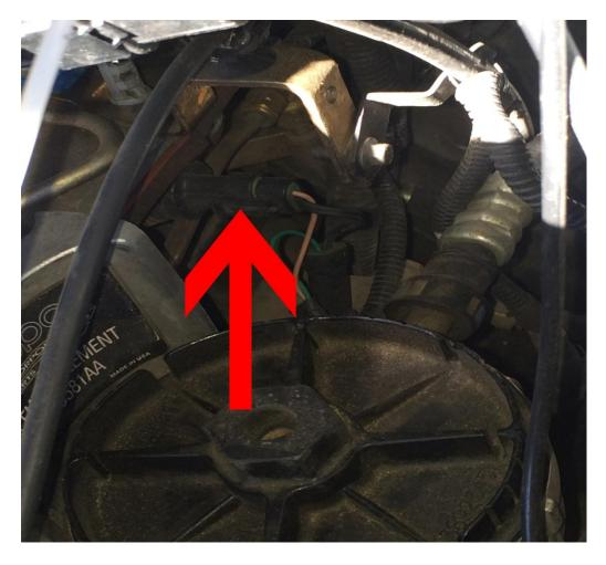
The MAP sensor is located on the driver side of engine, directly behind the factory fuel filter towards the firewall.
