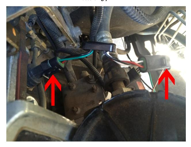
After you have plugged the factory harness into the Boost Fooler you are done! As stated earlier the Boost Fooler was designed to be "Plug and Play" for a simple and fast installation.
