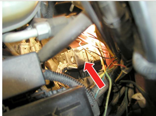
3. Once the cover is disconnected from the engine side of the computer the module can be uninstalled by pulling the computer towards you from inside the cab. Once the computer is removed the terminal where the chip installs will need to be cleaned (*thoroughly*) to remove the wax covering. The wax covering on the terminals must be fully removed for the chip to function. (*Shown in vehicle for demonstration only – remove before cleaning terminal*)
