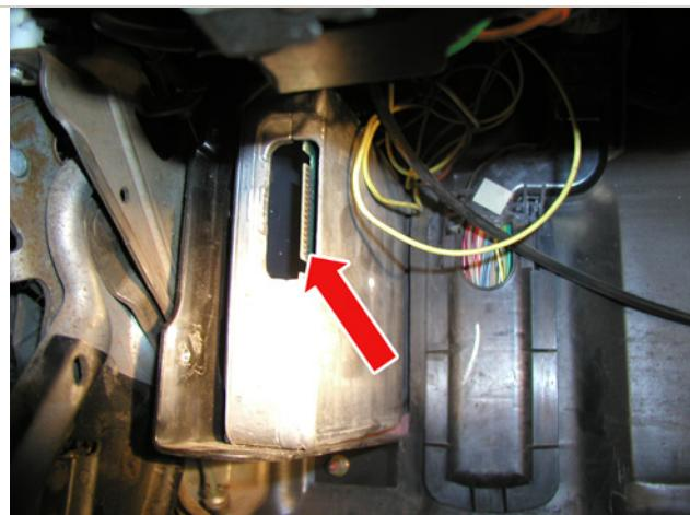
\* After the computer is removed you will be able to locate the catch code, which is needed to program the chip when ordering.
