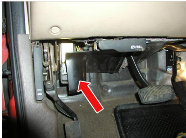
2. On the driver-side of the firewall in the engine compartment locate the plastic cover and wiring harness that covers the computer and disconnect it. There will be one bolt that holds the computer in place.
