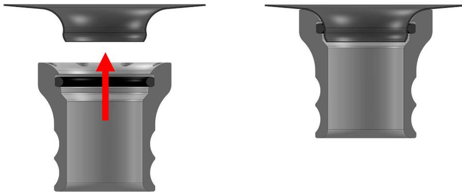
Lubricate the o-ring with clean transmission fluid. Slide the pickup tube directly onto the bottom of the filter.
