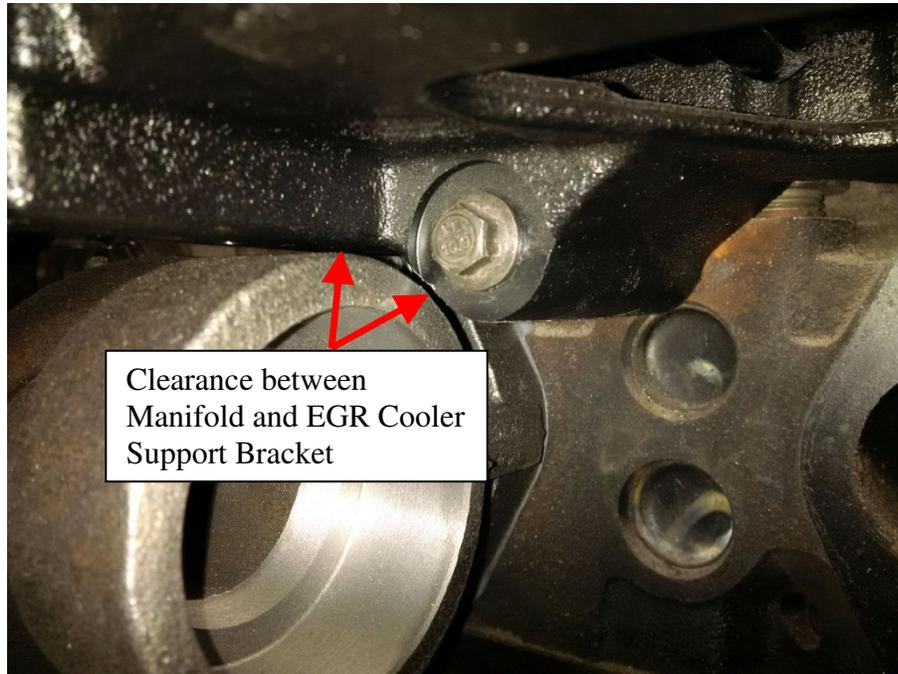
48. Line up the holes on the support bracket and reinstall bolts hand tight.
