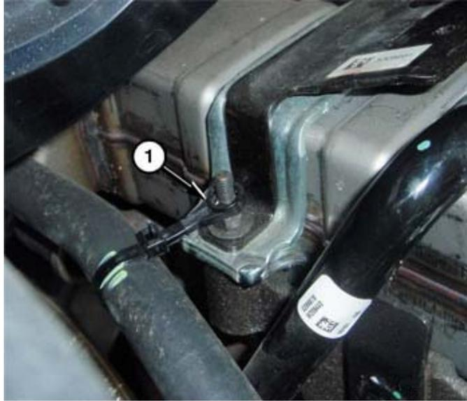
17. Remove the forward coolant tube from EGR cooler.
