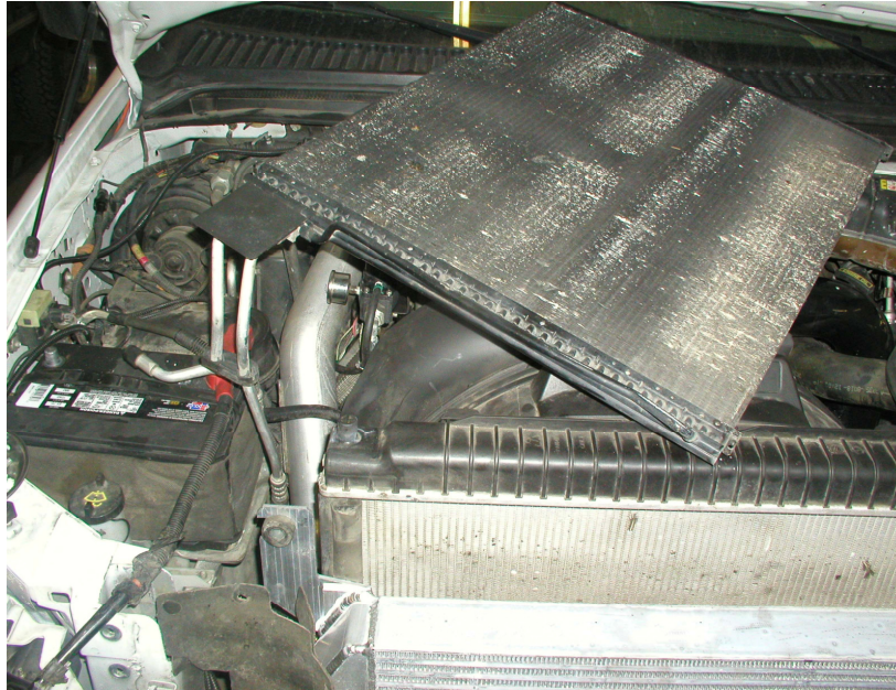
Figure 2 - Moved A/C Condenser
