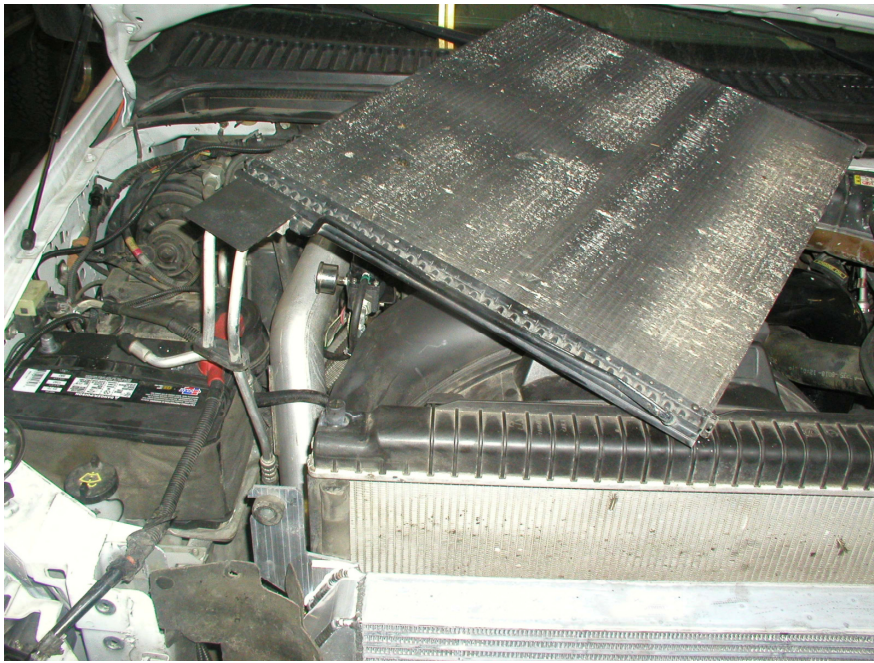
Figure 10 - Moved A/C Condenser
