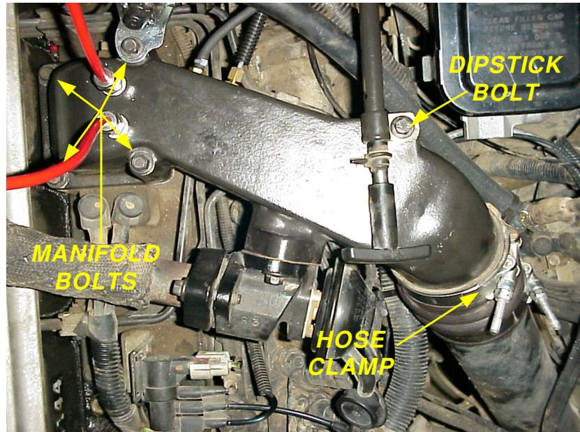
**Figure 2 - Dodge 12V Intake Manifold (shown)**
