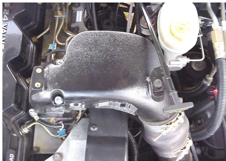
**Figure 4 - Arc-Flow Intake Manifold After Installation**
