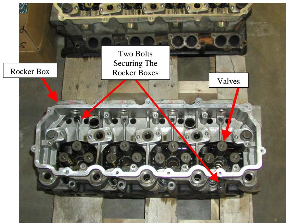
**Figure 1: Correctly Prepared Heads**
