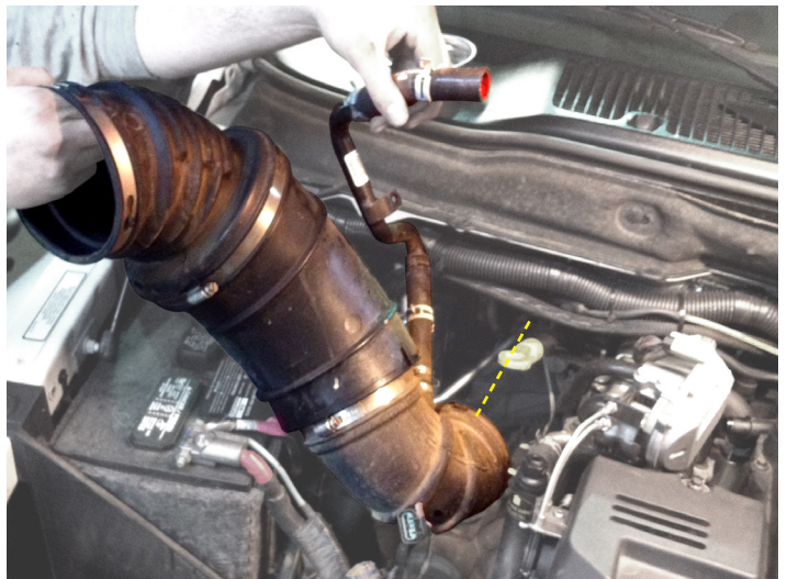
Loosen the hose clamp holding the intake tube to the factory turbocharger. Remove the crankcase breather tube and intake tube as shown
