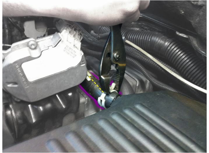
Disconnect the crankcase vent tube from the valve cover by moving the spring clamp show off the barb on the valve cover.
