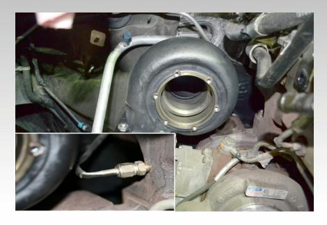
30.) LOOSELY INSTALL TURBO CARTRIDGE, (PN 01,B FIG.1) INTO TURBINE HOUSING. (EXHAUST HOUSING) CLOCK OIL DRAIN TO CLEAR VGT MODULE HEAT SHIELD AND TIGHTEN BOLTS OR CLAMPS AT TURBINE HOUSING. INSTALL OIL DRAIN LINE WITH PROVIDED HOSE CLAMP.
