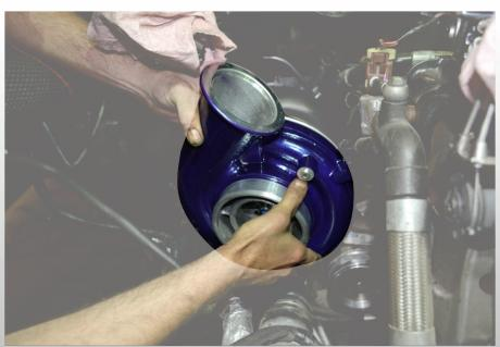
35.) PLACE SUPPLIED O-RING **(PN 21 FIG. 1)** IN CHARGE PIPE **(PN 3 FIG. 1)** TO FLANGE. INSTALL PROVIDED CHARGE PIPE INTO LOWER BOOT FIRST. THEN CLOCK TURBO AND ALIGN BOTH FLANGES TOGETHER. LEAVE BOTTOM BOOT LOOSE TO ALLOW BETTER ALIGNMENT OF CHARGE PIPE AND COMP HOUSING.
