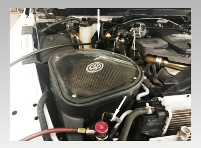
2.) DISCONNECT BOTH BATTERIES. REMOVE PASSENGER SIDE BATTERY. REMOVE TOP HALF OF AIR BOX AND INTAKE DUCTING.
