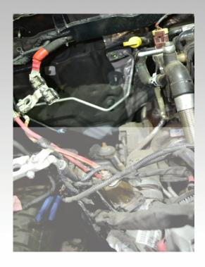
11.) DISCONNECT AC LINES AT FIRE WALL AND REMOVE THE LINE THAT RUNS FROM THE FIREWALL TO THE AC COMPRESSOR.
