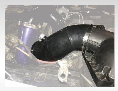
43.) INSTALL 90\* BARB FITTING INTO INTAKE BOOT. RECONNECT CCV LINE WITH PROVIDED HOSE. (PN 9,38 FIG.1)
