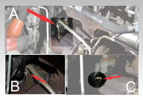
13.) LOOSEN AND REMOVE V-BAND CLAMPS ON BOTH SIDES OF TURBO OUTLET ELBOW. PENETRATING OIL MAY BE REQUIRED TO AID IN CLAMP REMOVAL.
