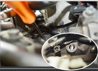
APPLY SMALL AMOUNT OF OIL TO O-RINGS BEFORE INSTALLING IN FREEZE PLUG PORT.
