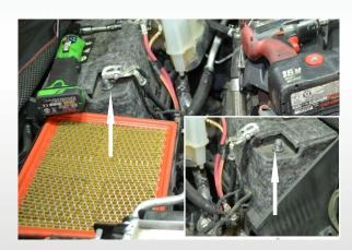
3.) DISCONNECT ACTIVE AIR WIRE HARNESS AND REMOVE WITH AIR BOX.
