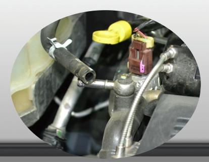
10.) REMOVE COOLANT RESERVOIR FROM FIREWALL.
