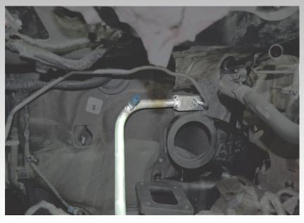
32.) NOTE CLEARANCE AT HEATER CORE HOSE. REMOVE HOSE CUT ½"OFF END OF HOSE AND REATTACH.
