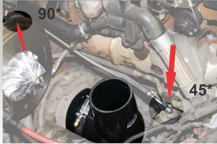
34.) INSTALL COMPRESSOR HOUSING AS SHOWN.(PN 01,C FIG.1) NOTE CLEARANCE AT COMP HOUSING AND OEM DRIVE PRESSURE SENSORTUBE. BEND TUBE AS NEEDED TO CLEAR COMP HOUSING.
